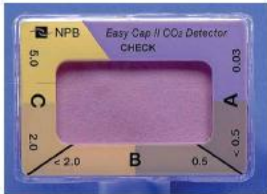
Figure 13. End-tidal CO 2 detector before application. The indicator is purple, which indicates failure to detect CO 2 . This also is the appearance when the esophagus is intubated.
